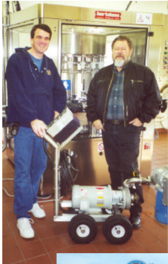
Fristam FT Series pump on cart does the job of three, and saves time.
