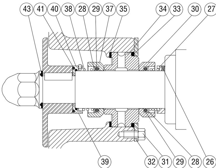
Figure 13: Double Seal Assembly
