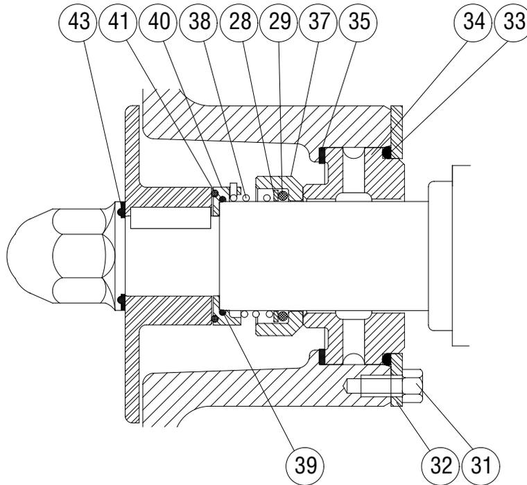
Figure 12: Single Seal Assembly
