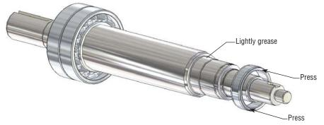
Press the outer race of the front bearing into the bearing block.
