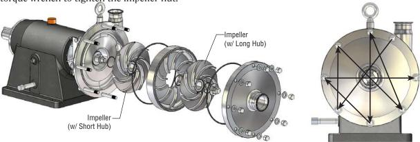
Prior to disassembling the bearing block, complete the pump head disassembly (Figure 8-10, page 16).
