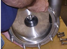
To remove the stationary seal and the flush seal components, the pump housing needs to be removed. Remove the four pump housing bolts and lock washers, which attaches the pump housing to the bearing block, using a 3/4" wrench. Carefully slide the pump housing off the end of the pump shaft, ensuring that the stationary seals (which are mounted in the pump housing) do not contact the pump shaft.
