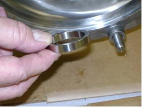
Align the pins on the rotating seal with the grooves on the seal driver and press the two components together. Wipe the seal face clean with a clean, soft cloth. Slide the gapping spacer onto the pump shaft. Note: it is important to use the same gapping spacer that was removed, as this is unique to your pump. This gapping spacer is what established the proper gap behind the impeller when the pump was assembled at Fristam.
