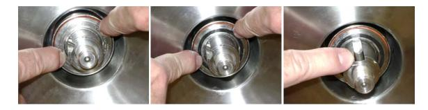
Lubricate the impeller gasket and place it into the groove on the seal driver. This gasket seals on the back side of the impeller. Place the impeller key into the shaft keyway.
