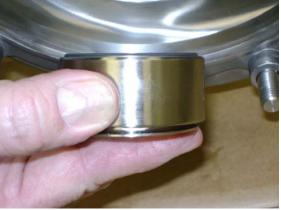
Lubricate the new seal driver o-ring and place it on the shoulder in front of the rotating seal. Note: This o-ring can alternately be placed on the pump shaft, up against the gapping spacer.
