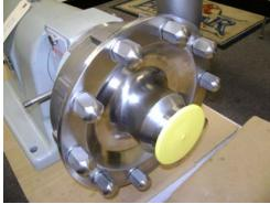
Model FPH3542 with double mechanical seal. Remove cover nuts with 1" wrench. Remove flat washers.
