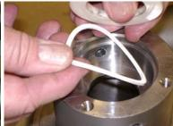
To remove the flush seal components, turn the housing over and place it on the housing studs. Remove the four retaining ring bolts on the housing with a 7/16" wrench. Remove the retaining ring, stationary water seal and flat gasket from the housing.
