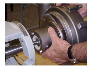
Carefully slide the pump housing over the pump shaft and push it against the bearing block, ensuring that the stationary seals (which are mounted in the pump housing) do not contact the shaft. Note: the stationary seals may be damaged if they make hard contact with the pump shaft.
