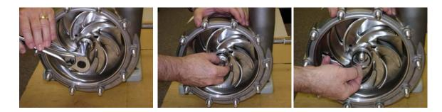
Place a chain wrench on the pump shaft near the coupling to keep the shaft from rotating while loosening the impeller nut with a 15/16" socket wrench. Remove the impeller nut and impeller gasket.
