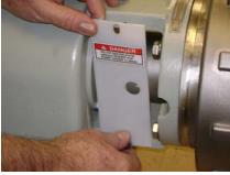
Remove the two water pipes from either side of the pump housing. Loosen the four guard screws and remove two plastic shaft guards from either side of the pump bearing block.
