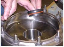
Place the pump housing on its hub. Remove the stationary seal by placing your fingers on the ID of the stationary seal and pulling it toward the front of the housing. The stationary seal o-ring should come out with the stationary seal.
