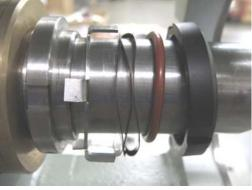
Now remove the rotating water flush components from the pump shaft, which include the rotating water seal ring, the water seal o-ring, the water seal spring and the water seal drive ring. The water seal driver may be left on the shaft.
