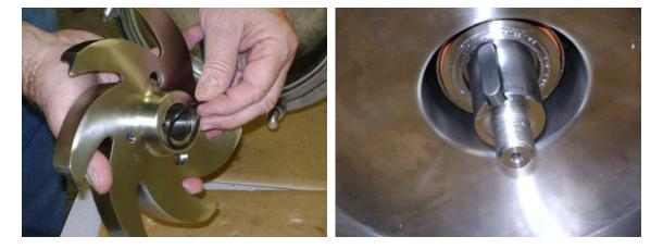
Remove gasket from back of the impeller, if it sticks to impeller. This gasket may stay positioned in the groove of the seal driver. Remove impeller key from the pump shaft.
