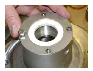
Replace the retaining ring onto the hub of the housing and install the four retaining ring bolts. Tighten with the 7/16" wrench to 4.5 ft.-lbs.
