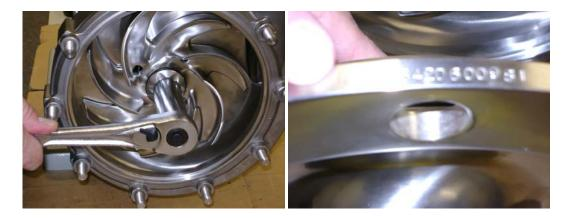
Place the chain wrench on the shaft near the coupling to keep the shaft from rotating while tightening the impeller nut with the 15/16" socket wrench. Tighten to 40 ft.-lbs. The picture at the right shows the pump serial number stamped on the side of the cover. Align this serial number with the matching serial number that is stamped on the pump housing when assembling the cover to the housing.
