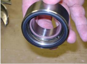
Slide the rotating seal assembly onto the shaft so the face of the rotating seal meets the face of the stationary seal.
