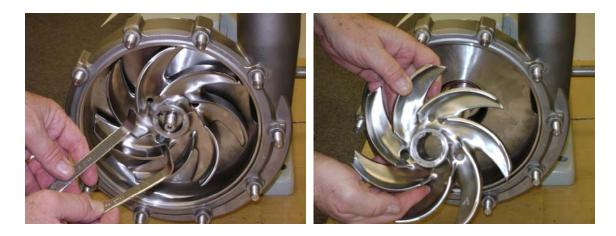
Remove the impeller from the pump shaft. Use impeller pullers to assist in removing the impeller, as needed. Be careful not to damage the threads on the end of the pump shaft.
