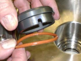
Turn the housing over and place it on the housing hub. Lubricate the stationary seal o-ring and place it on the new stationary seal. Place the stationary seal and o-ring into the bottom of the pump housing. Align the notch in the stationary seal with the pin in the housing. Press the stationary seal into the housing until it snaps into place. Wipe the seal face clean with a soft cloth to remove any oil or grit.
