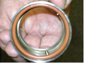
Place the new rotating seal spring into the rotating seal between the pins and the front seal face. Lubricate the new rotating seal o-ring and place it inside the rotating seal.
