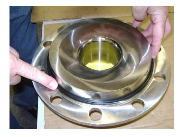
Place a new cover gasket on the pump cover. Note: you may need to stretch the cover gasket so that it fits more easily on the cover. The cover gasket needs to be ordered separately from the seal kit.
