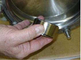
Remove the rotating seal assembly which includes the impeller gasket, seal driver, rotating seal, seal spring, and rotating seal o-ring. To remove this assembly from the shaft, place the impeller pullers on both sides of the assembly and pull toward the end of the pump shaft. Be careful not to drop this assembly as the seal face could be damaged.
