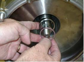
Remove seal driver from the rotating seal. Remove the seal driver o-ring from the shaft, then remove gapping spacer from the shaft. Do not discard the gapping spacer as it will be reused during reassembly.
