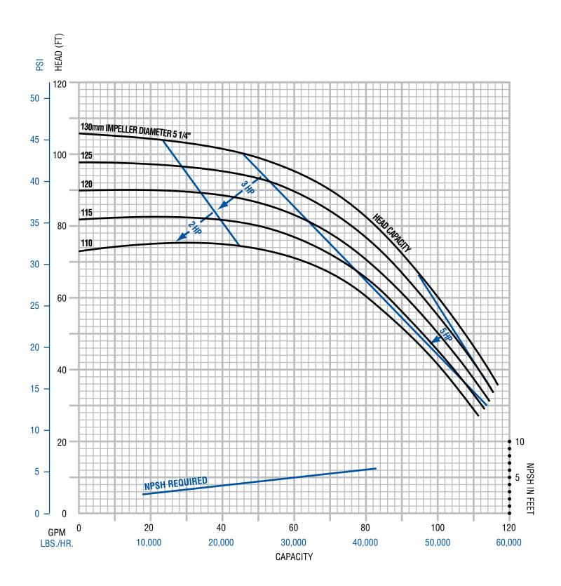
Performance curve based on tests using  $70^{\circ}F$  water and 0 psig inlet pressure. A tolerance of  $\pm$  5% applies to all figures. Actual performance may vary by application product. Please contact Fristam for different conditions.
