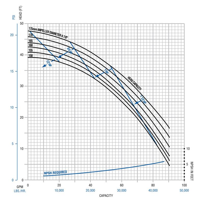
Performance curve based on tests using  $70^{\circ}$ F water and 0 psig inlet pressure. A tolerance of  $\pm$  5% applies to all figures. Actual performance may vary by application product. Please contact Fristam for different conditions.
