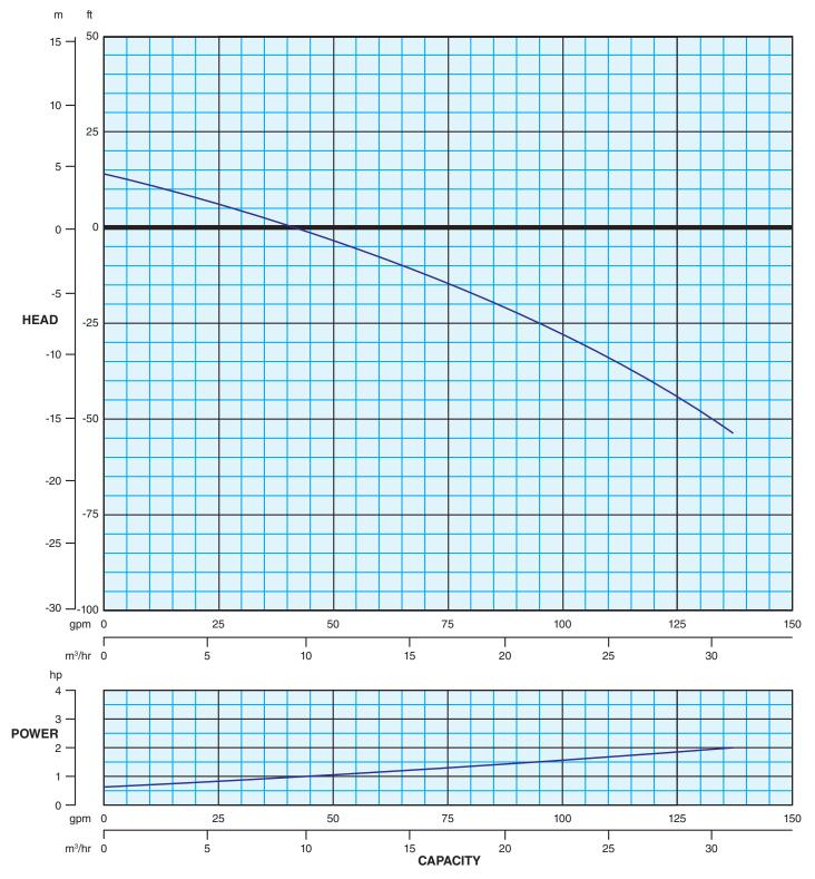
Curve based on tests using 70°F water fed by a centrifugal pump. A tolerance of  $\pm$  5% applies to all figures. Actual performance may vary by application product. Please contact Fristam for different conditions.
