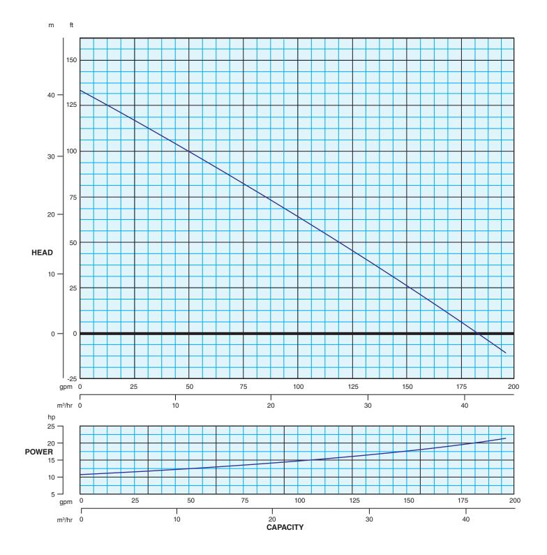
Curve based on tests using 70°F water fed by a centrifugal pump. A tolerance of  $\pm$  5% applies to all figures. Actual performance may vary by application product. Please contact Fristam for different conditions.
