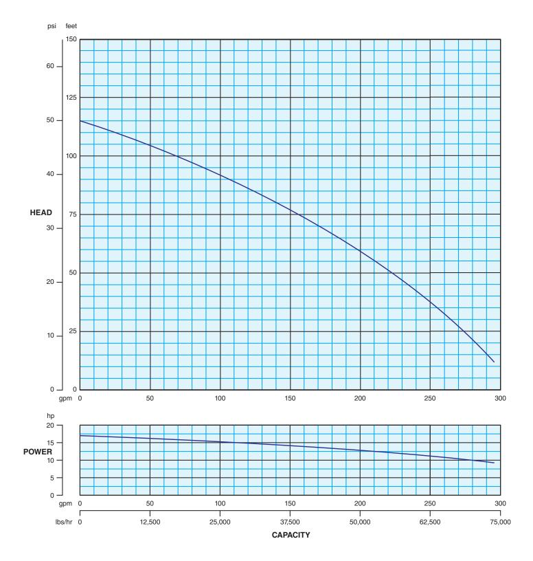
Performance curve based on tests using 70°F water and 0 psig inlet pressure. A tolerance of  $\pm$  5% applies to all figures. Actual performance may vary by application product. Please contact Fristam for different conditions.
