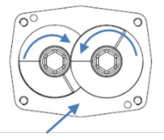
Laser marking indicates location of casing taper [view from front, cover removed]
