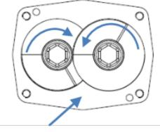
Laser marking indicates location of casing taper [view from front, cover removed]
