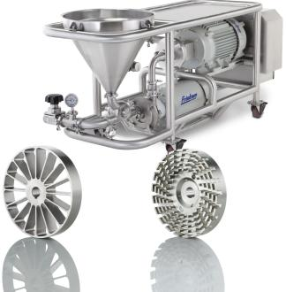
The Fristam Powder Mixer provides quick, highperformance blending of wet and dry ingredients into a fluid stream. It incorporates the uniform powder induction of the FZX liquid ring pump and thorough blending of the FS Shear Blender into a single, compact system. Powders can be wetted and dispersed on the first pass, dramatically reducing process times.
